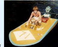
the power and immediately shifted his weight to the front and let the water rush in over the bow. The entire cockpit would fill up and the only thing you could see was the top of the motor gliding across the surface. Since the Mini Max could be made with sealed watertight compartments it was virtually unsinkable.
